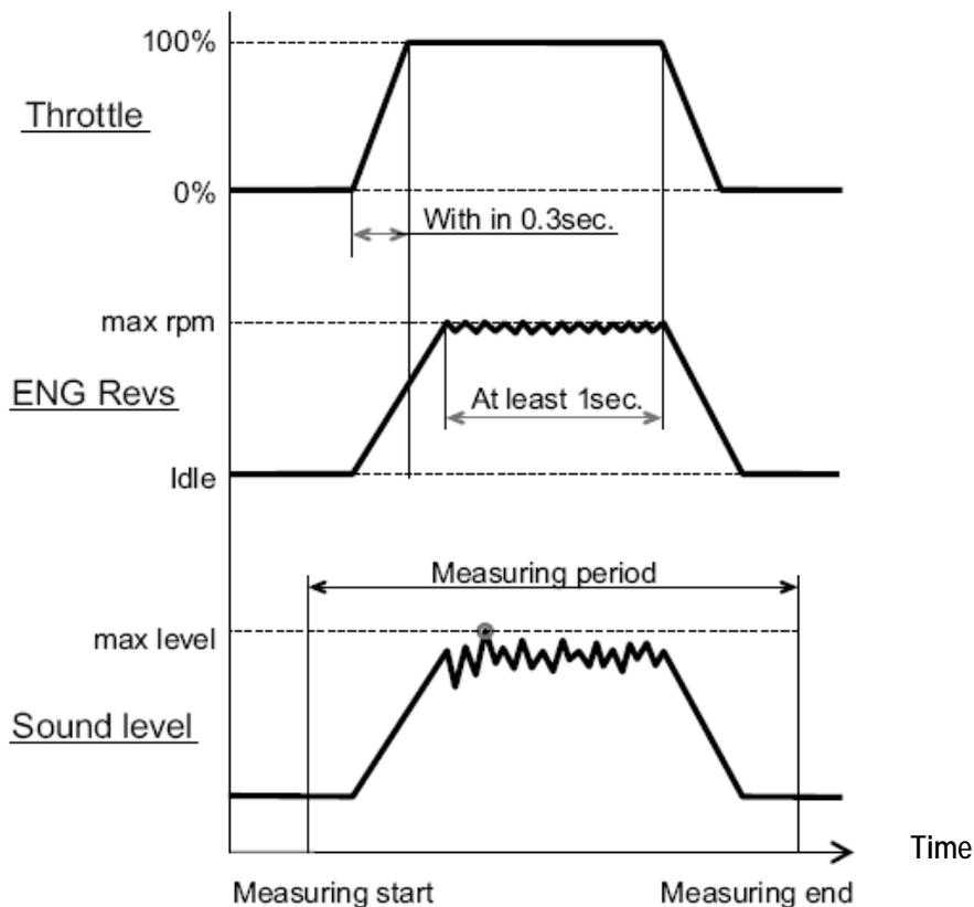
1. The Sound Control Officer shall open the throttle until full open throttle within 0.3 seconds.
