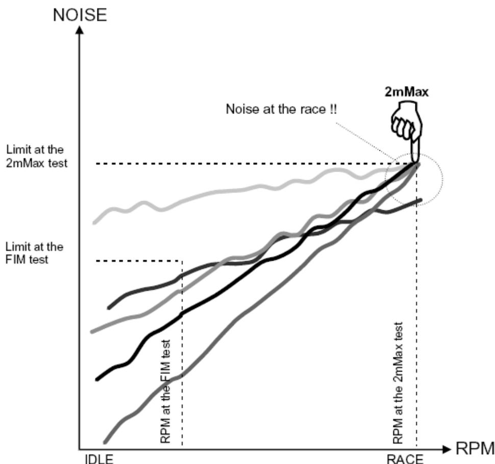
The "2 metre max" method will consist in quantifying not only the sound level produced by the silencer of the exhaust, but the maximum global sound level achieves by the motorcycle when the engine rpm's are raised to the maximum engine speed, limited by
